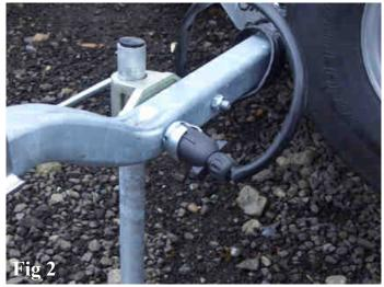
If fitting to the P6E 2004 trailer the storage bracket for the electrical socket must be removed and relocated to the chassis as fig 2. Ensure all bolts that have been removed are refitted and tightened fully.
