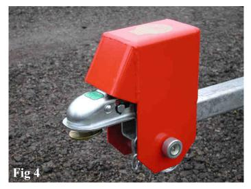
Lower the cover over the hitch handle. Insert lock bolt through both holes of the cover. Fit the recessed cup over end of lock bolt, then turn key a quarter turn to lock and remove key. Once lowered over the handle tilt bottom of Minilock slightly back. Fit the lock bolt behind the 'U' shaped stand. Fit the recessed cup over the end of the lock bolt and turn the key a quarter turn to lock and remove key.
