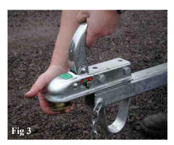
Insert dummy ball when trailer is un-hitched by lifting the hitch handle upwards and coupling in the normal way.
